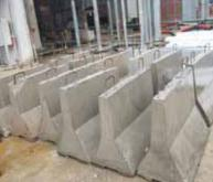
Surplus ready-mix concrete and concrete are used to repair road surfaces, build temporary road access, and fabricate concrete road barriers.
